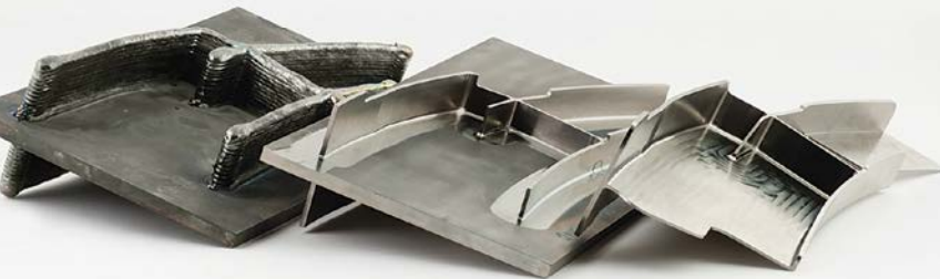
A Boeing 787 demonstration component shows (left to right) the part as printed, then the two machining steps required to produce the finished item.
